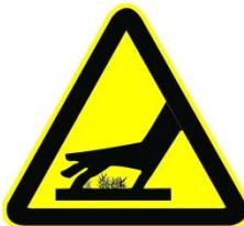
**Hot surface(s) present which may cause burns to unprotected skin or to materials which may be damaged by elevation**
