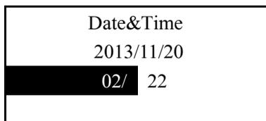
2. Press the set key S, to enter on the "time" setting. At this point the value part will be highlighted. Press the arrow keys to modify its value. Figure:
