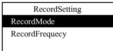
3. Press the Set key S to enter the storage mode setting interface. At this point the bottom line of the LCD screen can be set to options: Not stored, Timing, Alarm, and highlighted. Press the up and down keys to switch options. Figure:
